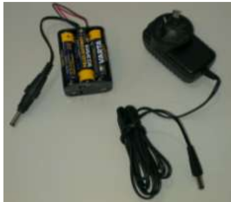
Fig. 23: Alternative power sources. We attached an old plug onto the battery pack. (If you do not have one available, we suggest simply wire the battery pack onto the back of the 2.1 mm socket. )
