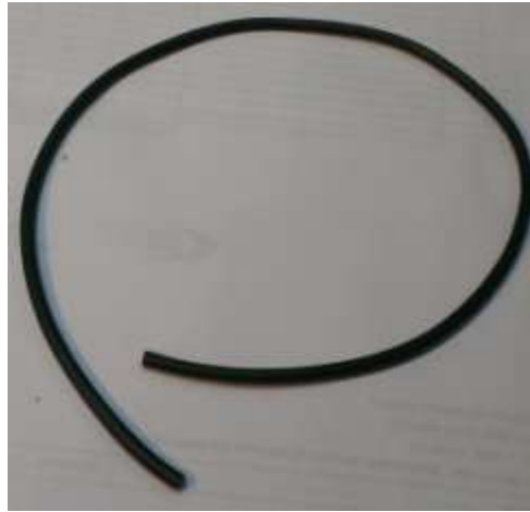
Fig. 7 : The shielded Audio cable as supplied with the kit.
