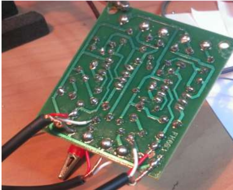
Fig 15: Showing the Volume control wires soldered to the underneath of the PCB. (Note: In this photo you can also see the Audio input wires attached to the pins on the top of the PCB)
