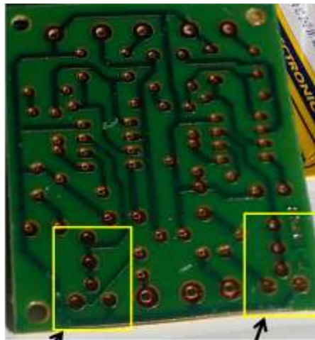
Right Volume Control and Left Volume Control connection Points for the cables.
