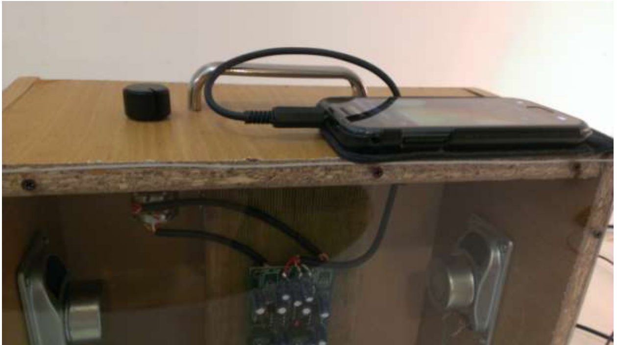
Fig. 25: Showing the volume knob seated close to the housing surface, along with a low cost carry handle.
