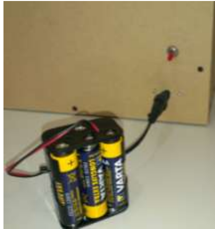
Fig. 24: Showing the ON/OFF switch and the battery pack plugged into the system.
