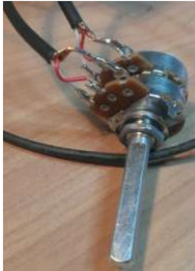
Fig. 9 : Showing the recommended orientation for connecting the Audio Cable to the Gang Potentiometer.
