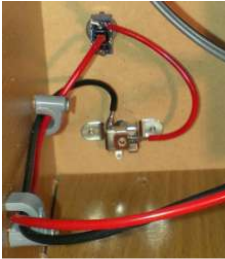
Fig 20: The power supply cabling, showing the Back of the 2.1 mm plug. The positive supply goes via a switch and then to the Amplifier.
