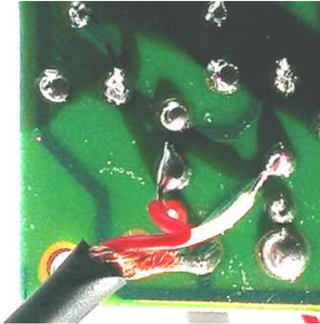
Fig 13: Showing wires soldered to the Right volume control points on the PCB. Note the white wire has been soldered to a point connected directly to the intended solder “pad”, but easier for us to access.
