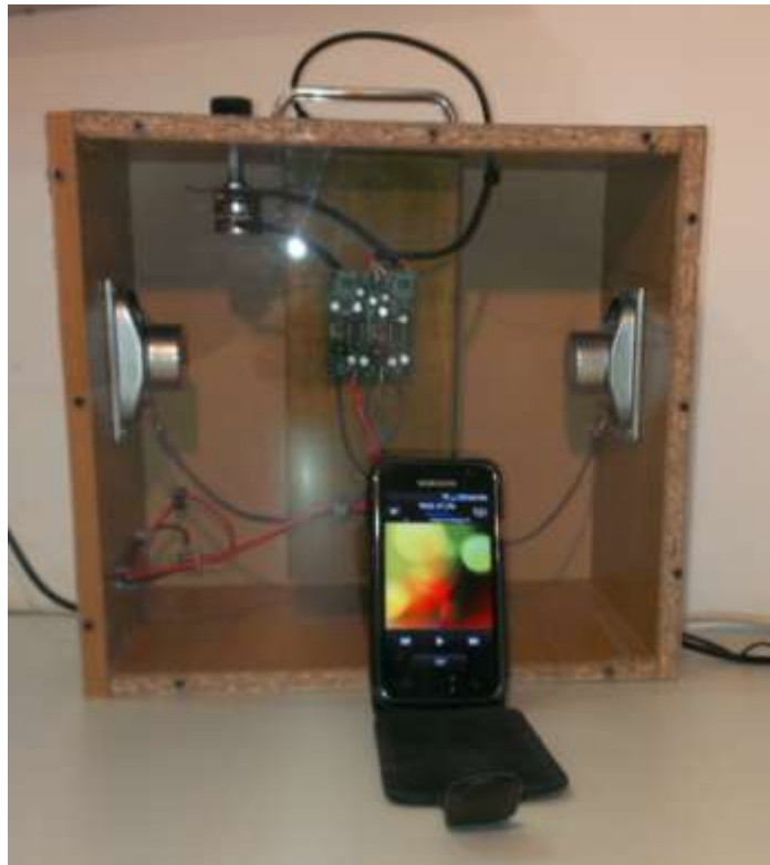
Fig 17: A demonstration housing made from scrap materials but which still gives a dramatic effect. (The clear front cover is to show the key system components).
