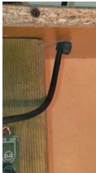
Fig. 22: Using a "zip-tie" for strain relief on the audio input cable.
