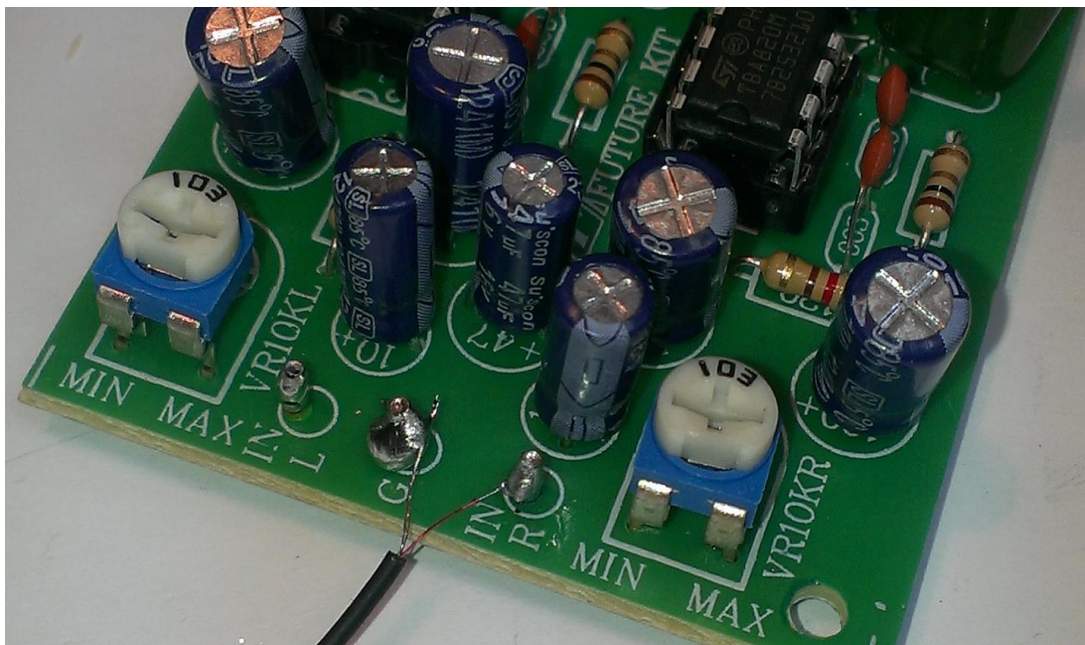
Fig 3.7 Showing the trimpots installed .
