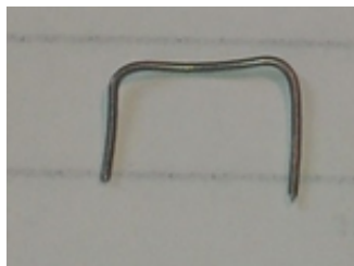
Fig 3.4 Study of the “Jumper” which we made from the cut off leg of a resistor. (Shown larger than real-life size).
