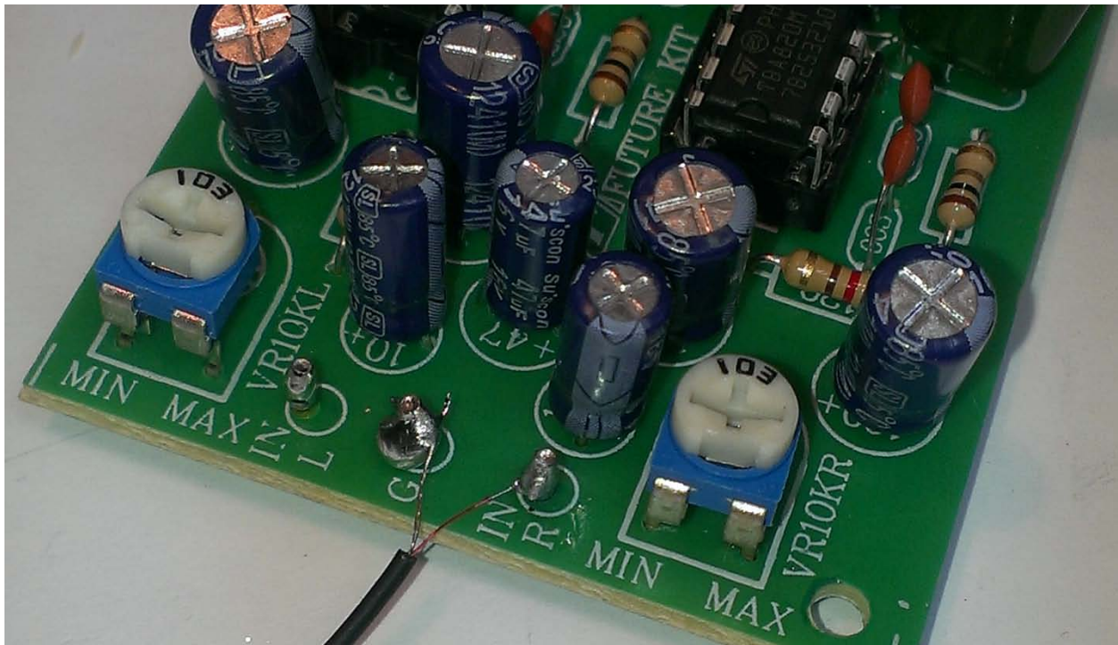
Fig 3.6 Showing the trimpots installed .
