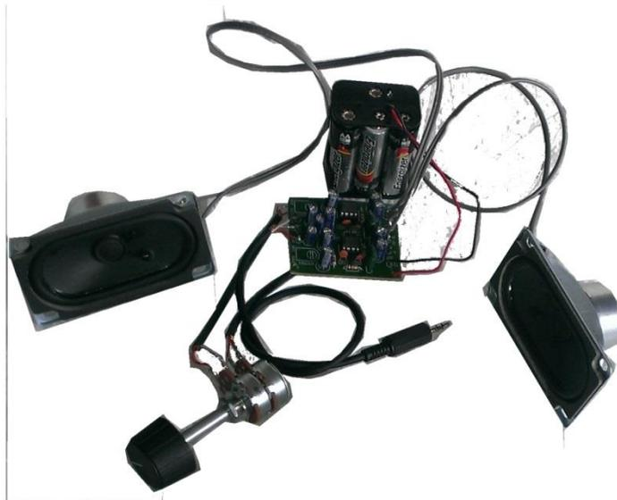
The key Electronics components of the 2-Watt Stereo kit.
