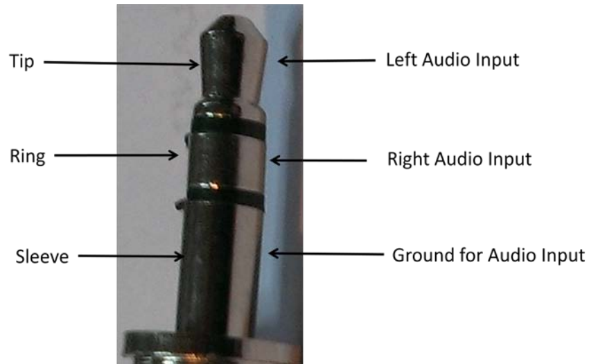
Fig 2: A close up of the plug and the different segments of it.
